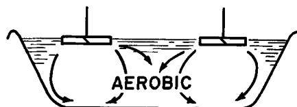
FIG. 3. A completely mixed aerobic lagoon.
